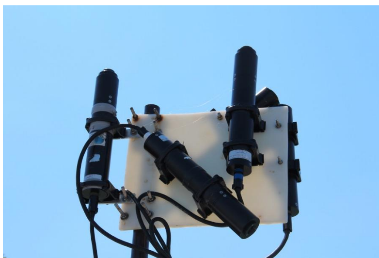
Fig.1: Radiometers used for the in-situ measurements in Lake Balaton.
