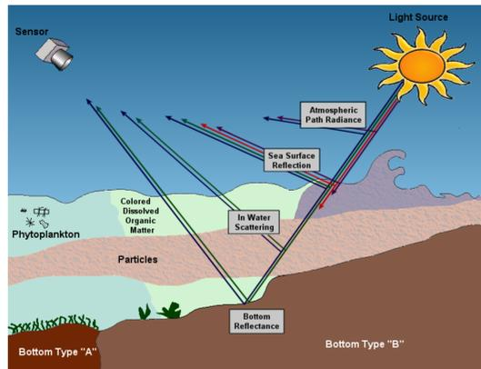
Detailed physical modeling is required to retrieve water inherent optical properties, bathymetry, bottom type, and other environmental products
