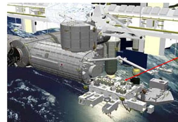
Experiment location for HICO on the Japanese Experiment Module – Exposed Facility
