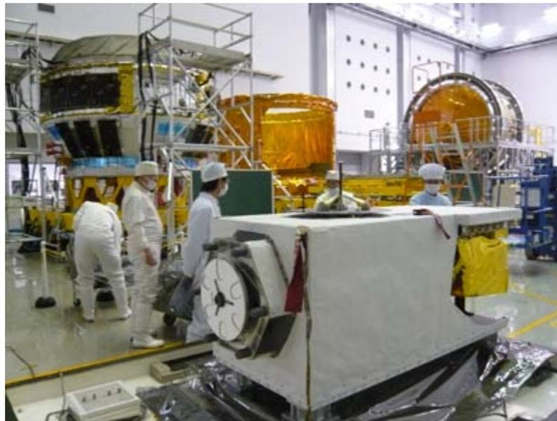
The HICO-RAIDS Experiment Payload (foreground) being prepared for installation aboard the JAXA H-II Transport Vehicle module (background).
